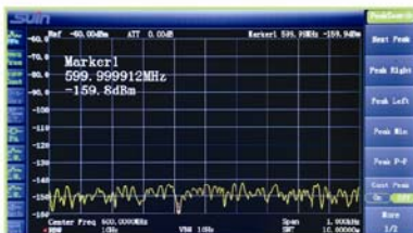
Featuring a low DANL of typ. -145dBm, distinguish two nearby signals clearly with 10Hz RBW
