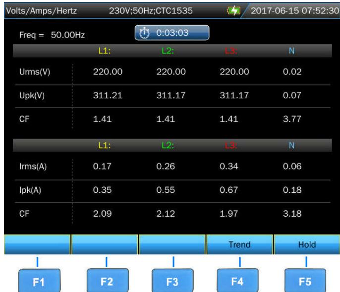
Table screen gives an instantaneous overview of important numerical measuring values under **Volts/Amps/Hertz** mode.
