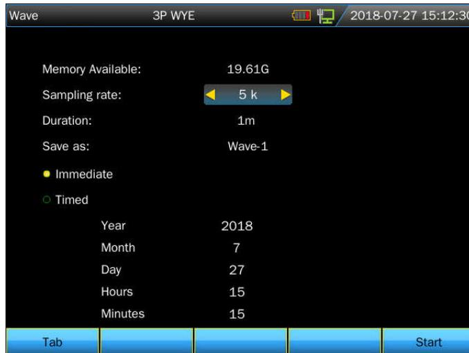
The file with WAV format could be generated after finishing recording and user could review it through PC software.
