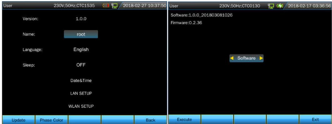
There are three types of update file including Software, Firmware and System. Select you wanted files to update, the Analyzer will give prompt after finishing update, then plug out the U disk, power off the Analyzer then power on to complete the update.
