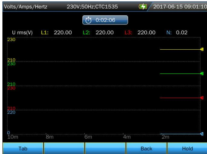
Trend screen shows the measurement value which is changing along with time change. Horizontal axis stands for the time, the Trend chart is forming from screen's right to left gradually.
