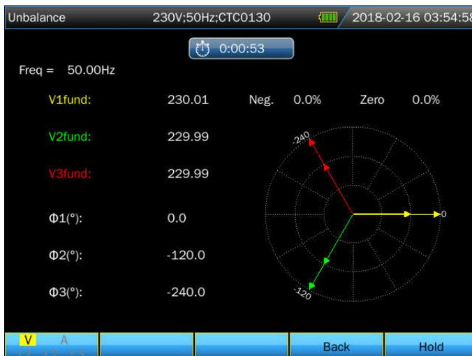
Shows the phase relation between voltages and currents in a vector diagram divided in 30 degree sections. The vector of the reference voltage **L1/A** points to the horizontal direction. Additional numerical values are given: negative voltage and negative current unbalance percentage, unbalance percentage of zero sequence voltage and zero sequence current, fundamental phase voltage and current, frequency, phase angles.
