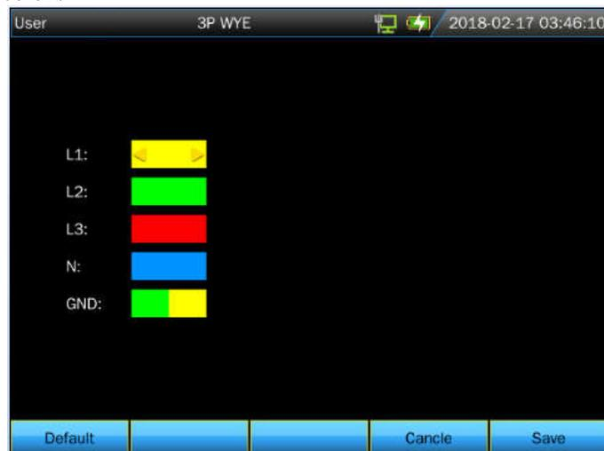
Press **【F2】** to set phase color according to local country standard for phase color definition. Different phase, different color, to represent measurement value of each phase. The default phase color settings of L1/A, L2/B, L3/C, N and GND separately are yellow, green, red, blue and green.
