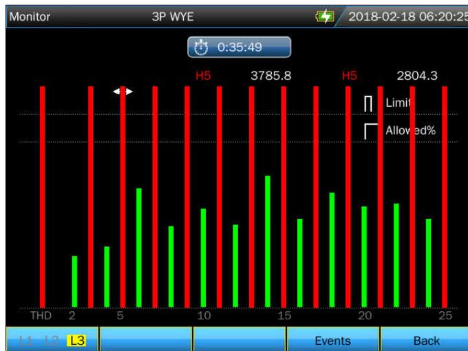
The main system monitor display shows the worst harmonic for each of the three phases. Function key **【F2】** brings up a screen with Bar Graphs showing the percentage of time each phase spent within limits for 25 harmonics and Total Harmonic Distortion (THD). Each Bar Graph has a wide base (representing an adjustable limit of e.g. 95%) and a narrow top (representing the limit of 100%). A Bar Graph changes from green to red if the limits for that harmonic are violated.
