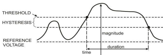
Fig. 3-3-2 Characteristics of a voltage swell
