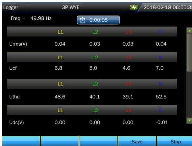
The table screen displays all the real time measurement data as selected parameters. With left/right key to refer to next page for view of the data.
