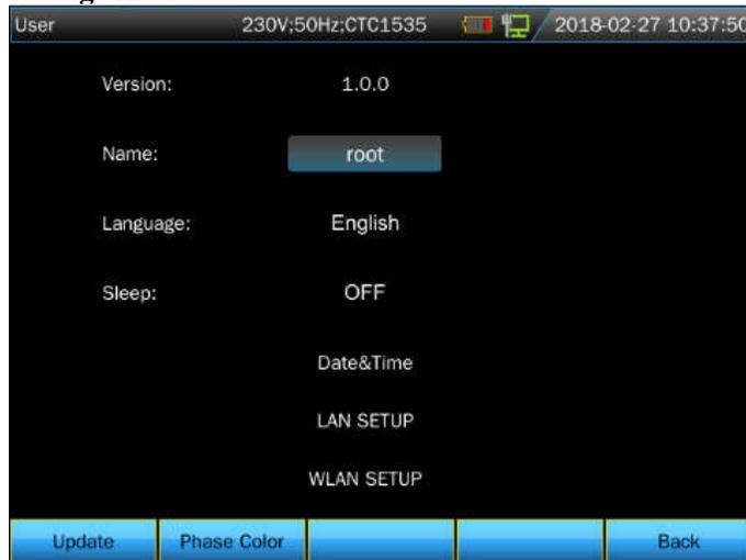
The user name, language, sleep time, system time, and network setting could be set in this interface by keys of **【▲】** **【▼】** **【◀】** **【▶】** and **【ENTER】** keys.
