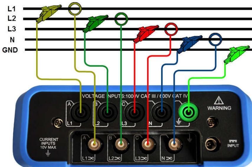
The Analyzer has 4 BNC-inputs for current clamps and 5 banana-inputs for voltages. For a 3-phase system, make the connections as above picture show.
