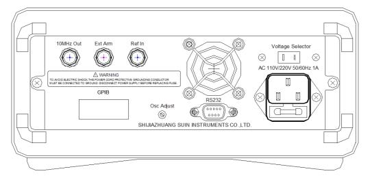
**Ref In** External frequency standard input, 5MHz or 10MHz can be selected, switch automatically inside the instrument.
