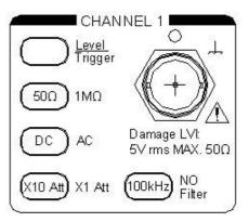
1) [Level/Trigger] key, press this key the indicator light on and the 'LEVEL:+0.000V' will be shown in the display, the value is adjustable. Then use the  $[\uparrow] [\downarrow] [\leftarrow] [\leftarrow] ]$  key to adjust the trigger level and press [Enter] to
