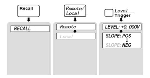
All function keys are transparent with green LED under. When function enabled or disabled, the corresponding LED will be lighted on or off. Please refer to next chapter for detail descriptions.
