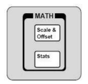
Note that Math and Limits are not available for Totalize and self-check measurements. As shown in left diagram, the keys of **[**Scale&Offset**]** and **[**Stats**]** are included in MATH function area. The MATH function is disabled in the initial state and the annunicators of the two keys are OFF.
